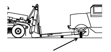
Block the axle or the tires. Return the FWTD to the original position and back under the truck for a normal pick.
