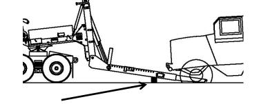
Place blocking under the booms to the rear of the boom cross-member.
