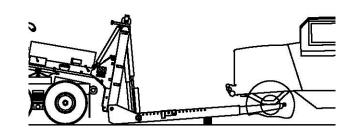
"Retract" the booms. The blocking allows the booms to act like a seesaw and will lift the axle of the truck.
