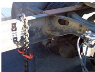
NEVER WRAP A CHAIN AROUND AN INDIVIDUAL FRAME FLANGE
