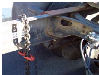
NEVER WRAP A CHAIN AROUND AN INDIVIDUAL FRAME FLANGE
