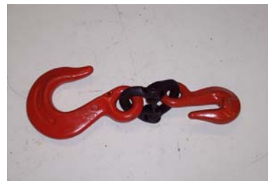
Sling Hook end to a suitable structural member. Grab Hook end to chain from boom extensions.
