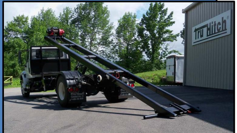
The hydraulic tail has a two position body pin lock. When used with a flatbed body, you can securely slide the body and load at a low 17° angle just like a rollback truck.
