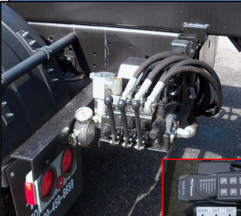
A three bank, filtered control station, with a six function wireless radio remote control, powers the 25K winch, the lift cylinders, and the tail extensions. When packaged with an automatic transmission you have complete control to work with the load on your terms.
