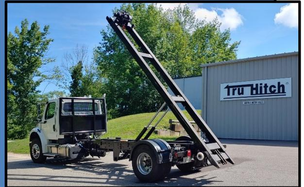
When extended, the 8' hydraulic tail extension of the Tru-Hitch Tilt Slider System creates 28' of hoist rail for controlled loading and unloading custom body configurations. The integrated folding ICC bumper travels with the extension.
