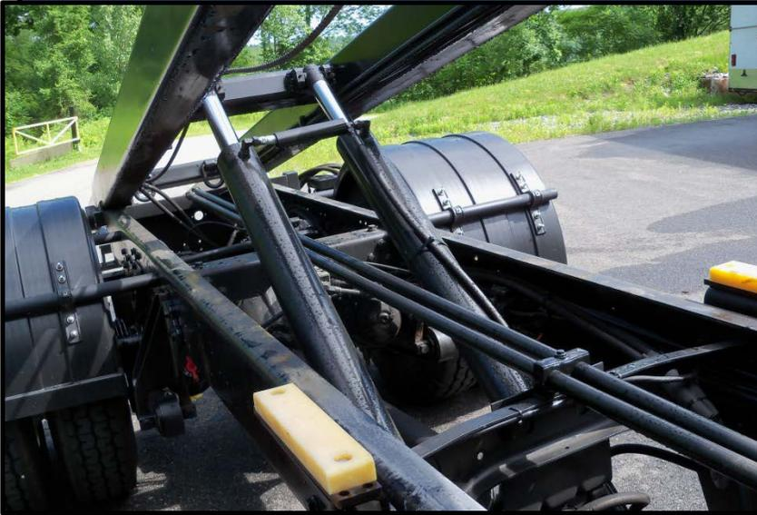
Twin 4.25" bore hydraulic cylinders with 54" of stroke provide 20,000 lbs of lift capacity at a dump angle of 50°
