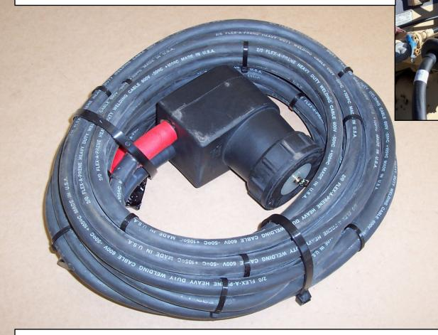
You should have this cable with the hitch. Take the big head off the cable and put the wires directly on your truck's batteries. The other end will plug into what was labeled the 24V receptacle of the box. ( you have converted it to feed 12V now)
