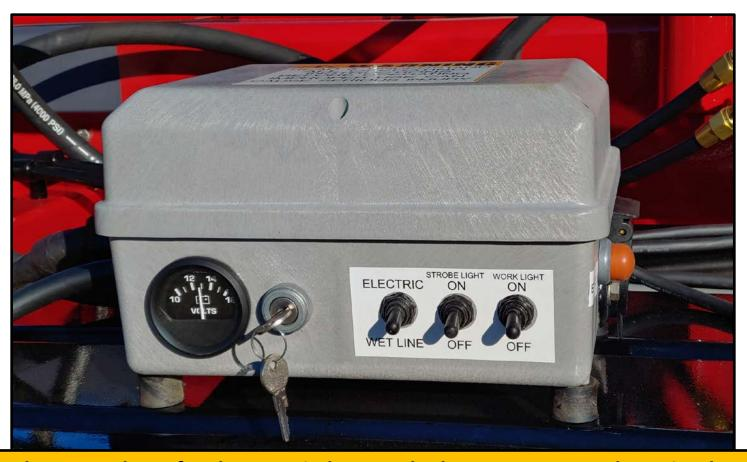
The Control Box for the Tru-Hitch. Turn the key on to power the unit. The "Electric"/"Wet Line" switch determines how the remote control operates in those modes, and the Strobe and Work Light switches operate onboard lighting. The voltmeter gives visual confirmation of battery condition and charging. The remote control receiver is connected to the Control Box.
