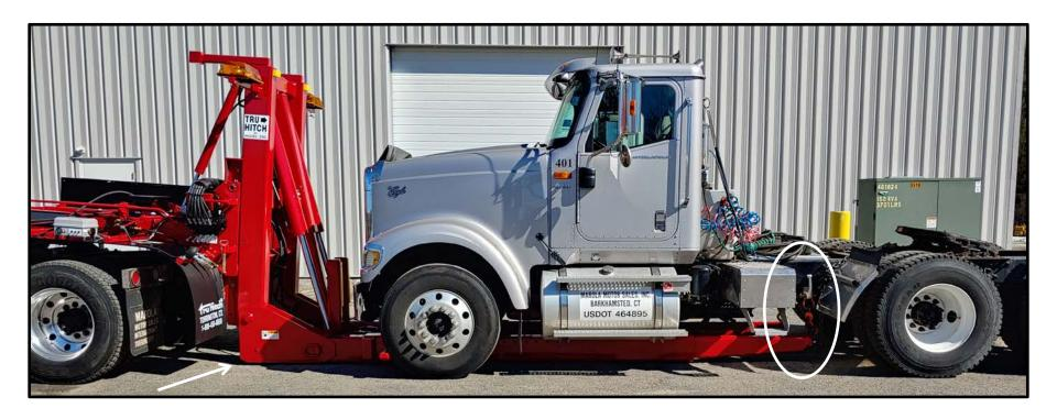
Once the rear hook up chains are in place, BOOM EXTEND slightly until the chains at the rear tighten, and the base of the boom at the mast comes slightly off the ground. We call this the "float" position. It will center the pick to your chaining setup. Check your rear chains to make sure the pull looks vertical and that nothing came loose.
