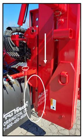
Once loose, remove the pivot pins and stow them in their holders. Then MAST RETRACT to bring the mast down and fully engaged into the fifth wheel section.
