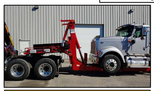
Now BOOM EXTEND until the hole in the center ram is exposed that will keep the fifth wheel level for towing. Insert the safety pin and BOOM RETRACT just enough to set the pin.
