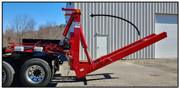
**BOOM RETRACT until they are** fully retracted against the mast.
