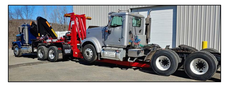
Truck is in the lift tow position, Fifth wheel area of tow truck is level, and safety pins are installed. The only place this load will pivot is at the fifth wheel. You have essentially turned the towed truck into a trailer! Only after you have the safety pins in place should you go under the axle area to install safety chains.
