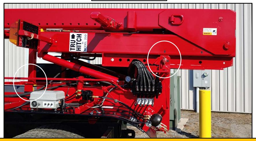
Just after the support arms contact the fifth wheel section the pivot pins will loosen. Once the pins loosen remove the two pins and place them back in their holders.
