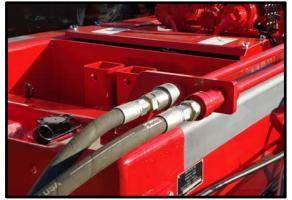
Wet Lines – 2. Connect the lines from the PTO to the hard line connections.
