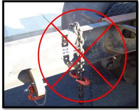
Here are other different methods to make a rear hook up, chain basketed over both sides of open frame to a clevis on end of extensions, chain directly around extension, or using the frame hook with chains. There are also sling hook/grab hooks provided to create chaining points. Use what is best for the situation. However NEVER wrap a chain around an individual frame piece. This could damage the frame.
