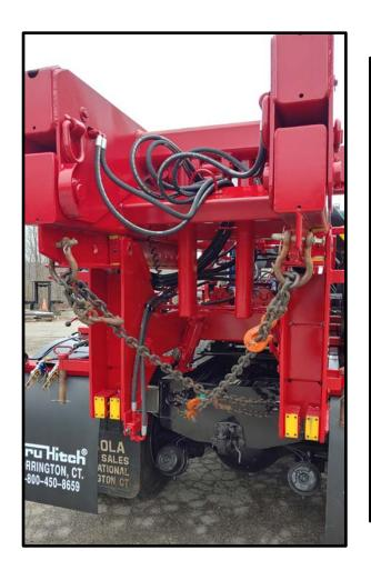
Finally, install a set of clevises in the end of the mast and then loosely install cross chains from the clevises to the rear of the frame on your tractor. Once installed, MAST **RETRACT** to tighten the chains. This will secure the Tru-Hitch from moving during transport.
