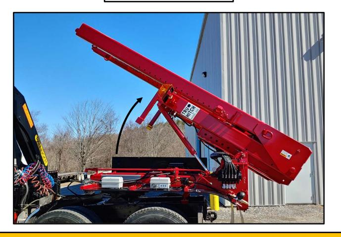
MAST EXTEND to bring the mast and booms to the vertical position.
