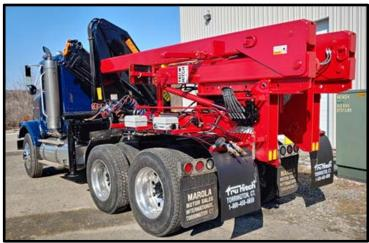
Once the pins are removed MAST EXTEND to bring the mast and booms over the fifth wheel. CAUTION – Do not extend past the second arrow or damage to the support arms may occur.
