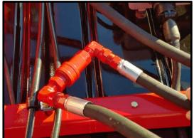
Wet Lines – 1. Remove the soft lines and connect them together
