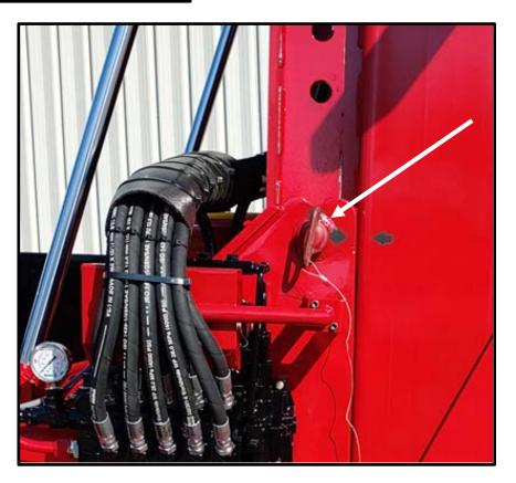
Remove two pins from their holders and insert them into the pivot holes on both sides of the hitch.
