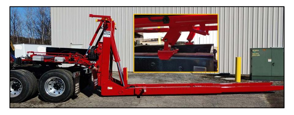
BOOM RETRACT to set the transport legs onto the frame of the tractor.
