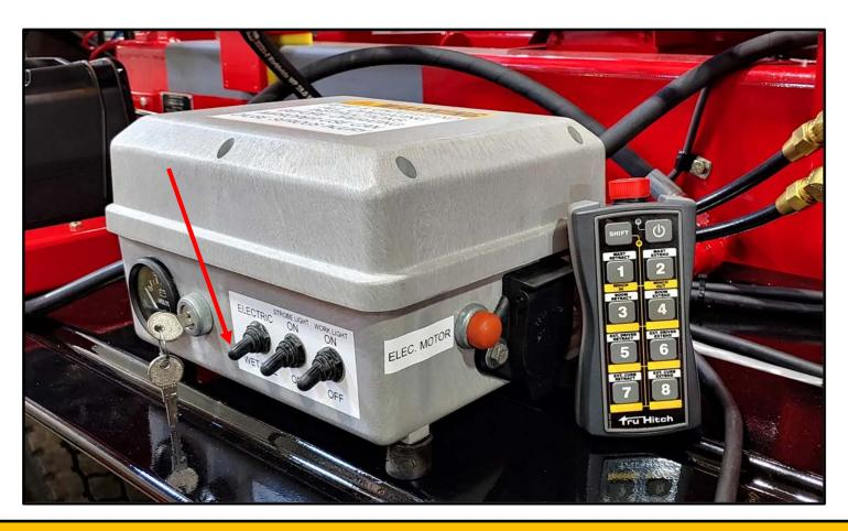
Make sure to set the Control Box to Electric or Wet Line to match how you are operating your hitch. When operating in Wet Line there is no need to press the electric motor button, and the remote control will operate the valve control levers without activating the pump motors
