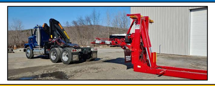
To attach the Tru-Hitch to your tractor simply align yourself to the front of the hitch, and then back until your fifth wheel is centered under the front of the fifth wheel section.
