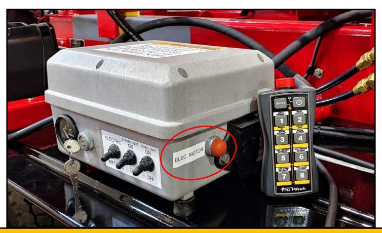
In "Electric" you must press and hold the orange button to activate the pump motors on the Tru-Hitch. If using the remote control in "Electric", the pump motors will activate automatically. If you are using PTO driven wetlines from your tractor the control box is set to "Wetline" and orange button is not used, and the pump motors will also be automatically deactivated during remote control operation.
