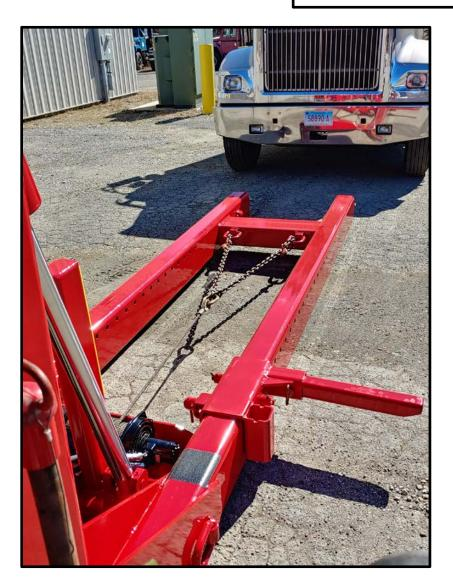
Line up to the truck you want to tow. Booms off the ground, just enough to back without dragging, while still allowing the booms to get under axle of truck you are towing. Adjust your receivers on the booms so that the wheel stops will contact the tires of the towed vehicle without the front of the vehicle contacting the bumpers stops on your Tru-Hitch.
