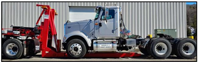
Now EXTEND the Extensions to an area that you can make a rear hook up with chains. Go as far back as possible for the truck you are towing. In this example, the area just forward of the rear axles is easy to get at for chaining. It will be different for each truck.
