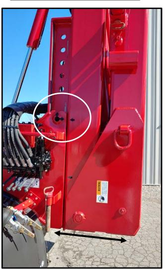
MAST EXTEND until black arrow on the mast aligns with the black arrow on the pivot hole of the fifth wheel section.
