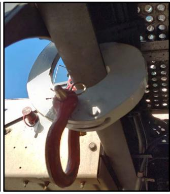
Now you make your rear connection from the truck to the Tru-Hitch. Here it shows a chain run between the twist clevises on the end of the extension and frame hooks. The frame hooks are made so that, when space permits, they can be rolled onto the frame whole or pinned after being placed into position.
