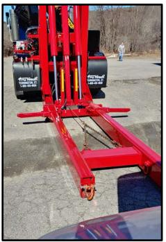
BOOM EXTEND until the booms are parallel to and just off the ground, ready to back under a truck.
