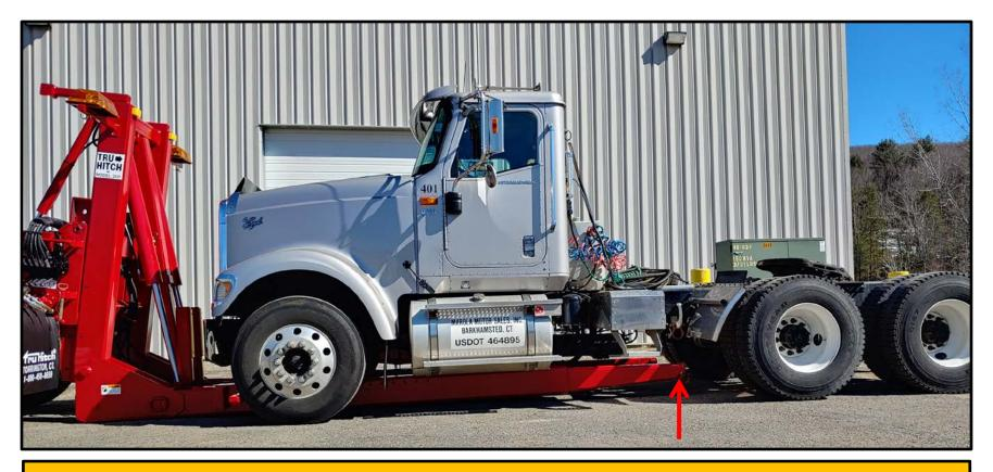
Once Transport legs are out of the way, BOOM RETRACT until the booms and extensions are as high off ground at the rear as possible, without hitting anything underneath the truck. (air tanks, fuel tanks, crossmembers, etc..) How high will vary by the pick but don't panic if you only get a few inches. That will be enough.
