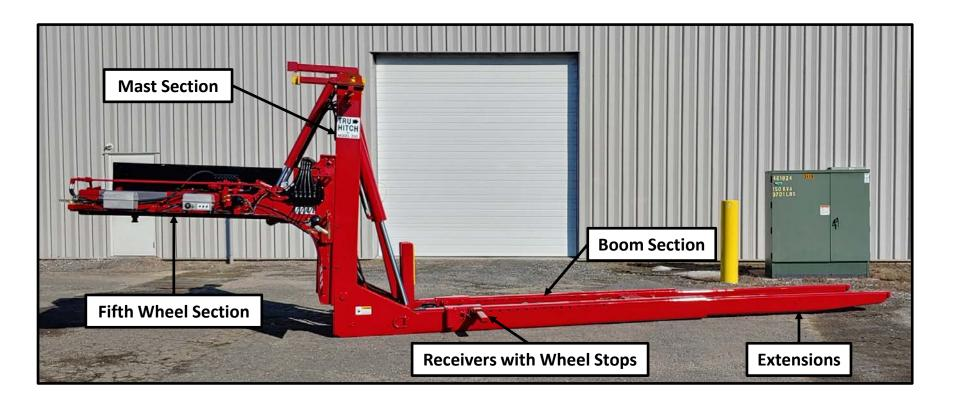
There are no permanent connections required to use the Tru-Hitch. A standard wheelbase tractor is all that is needed. When the Tru-Hitch is disconnected and parked with it's extensions out, it can sit safely ready to back a tractor under. It takes just a few minutes to connect to your tractor and place into transport configuration.
