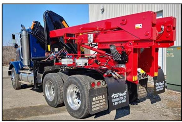
In preparation for lift towing from the transport configuration MAST EXTEND slightly to loosen your transport chains. Remove and stow the chains and clevises.
