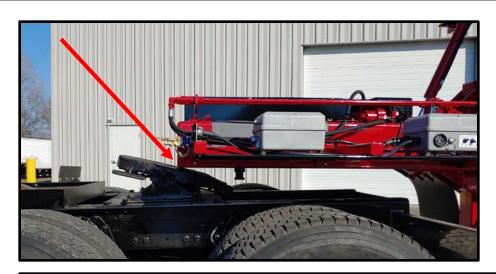
Use the Boom function to level the hitch, and the Mast function to adjust the height of the hitch to your fifth wheel, and then back under and lock into the Tru-Hitch just like backing under a trailer.
