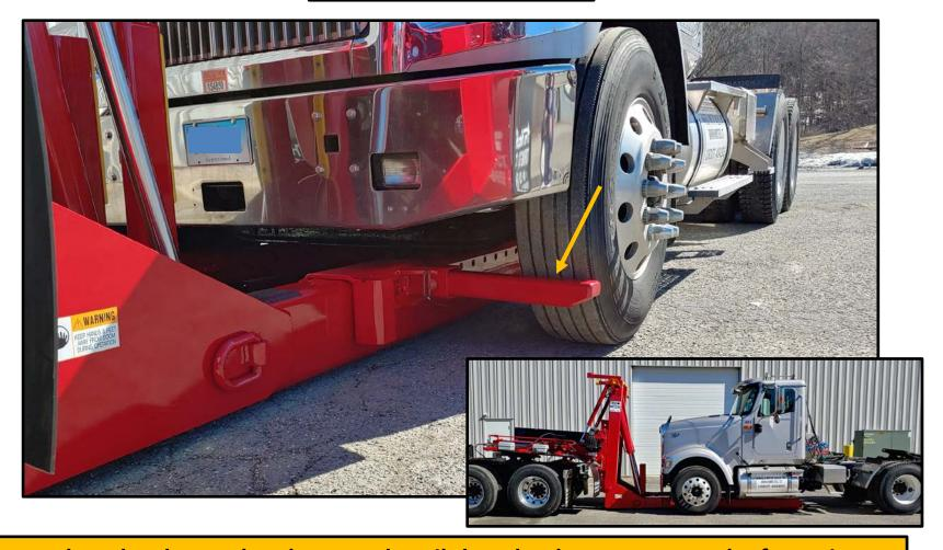
Back under the truck to be towed until the wheel stops contact the front tires. You want the wheel stops contact pattern to be as even as possible on both sides.
